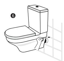
Before installation, fit the seat cover on EWC. Fit the W\M Ext. EWC in the bolts (fitted inside wall) and outlet rubber gasket on outlet of EWC for connecting with waste outlet. Tight the same & put chrome plated cap on the bolts and connect the water connection with the flexible connecting pipe.
