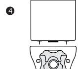
Place cup type rubber gasket at the bottom of beta valve and couple with W\M Ext. EWC with fly nut.
