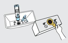
iii) Fit the beta valve in the central outlet hole & tight the checknut at the bottom of cistern.
