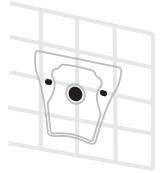
Fix the rag bolt with the help of sleeves & The outlet hole in the wall should be made as mentioned in (B).
